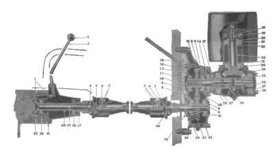
1 Fork and Rod ller 22. Shims 2. Ball 23. Spacer 24. Shims 3. Lever 4 Nut 25 Shims 5. Spring 26. Pinion 6. Button and Spring 27. Cone and Roller 7. Trunnion and Ball 8. Cup 28. Cup 29. Shaft 9. Bearing 30 Gasket 10. Snap Ring 31. Shims 11. Plate 32. Gasket 12. Gasket 33. Gear 13. Retainer 34. Shaft 14. Gasket 15. Gear 35. Gasket 36. Washer 16. Oil Seal 37. Oil Seal 17 Oil Seal 38. Ball Bearing
